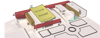
SUSTAINABILITY FEATURES A: VERTICAL LOUVERS B: HORIZONTAL LOUVERS C: ELEVATED CANOPY
