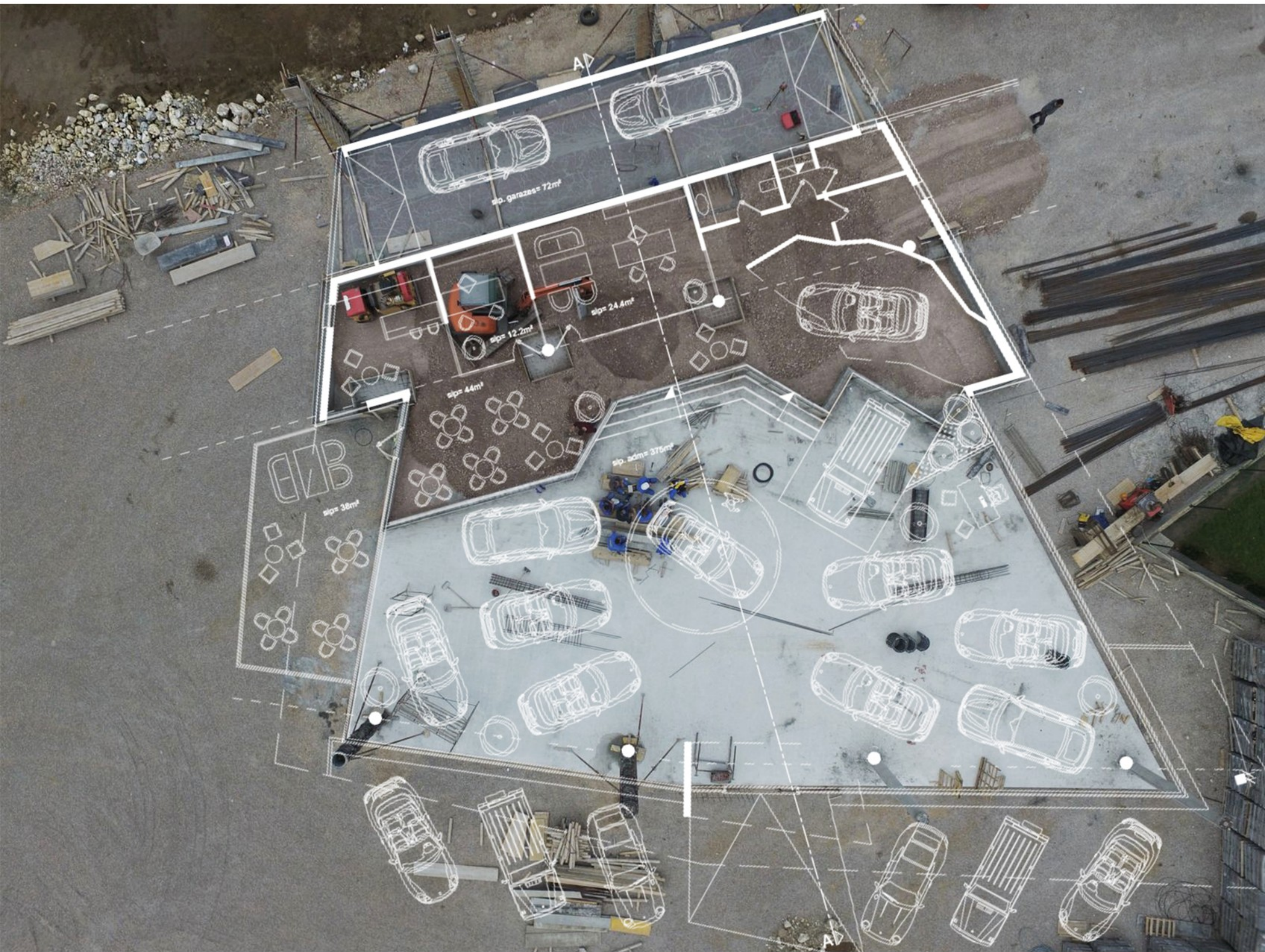
Site layout plan, set out on location during construction works
